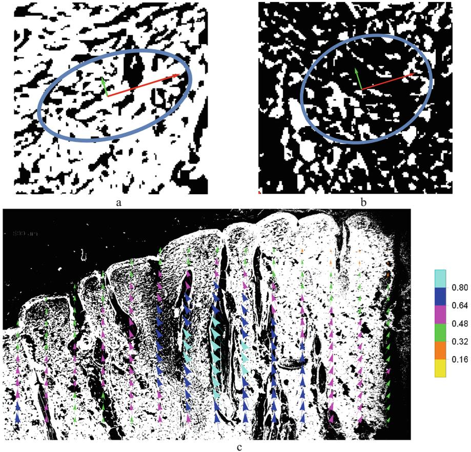
**Fig. 2.** Illustration of fabric tensor and its eigenvectors: a – fabric tensor in mesh element with aspect ratio 0.27 and density 90%, b – fabric tensor in mesh element with aspect ratio 0.80, density 68%, c – vector field normalized by aspect ratio with the origin bitmap.
